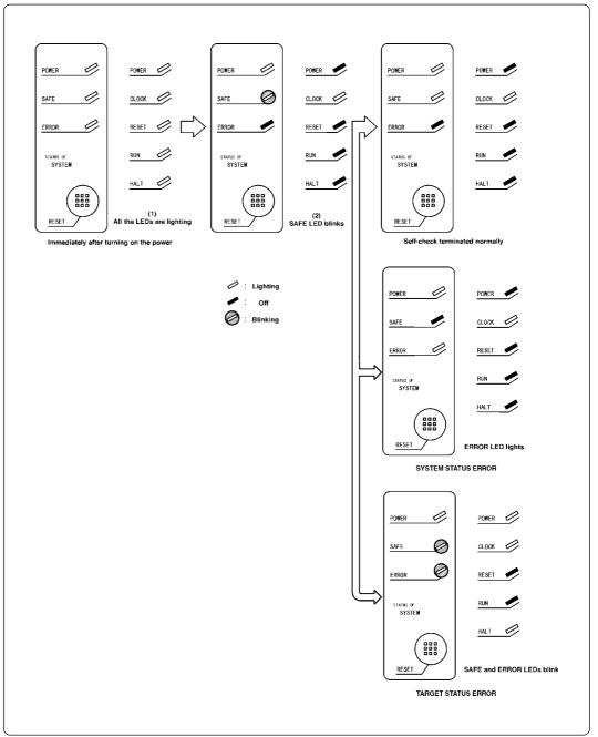
Figure 4.4 Self-check procedure
